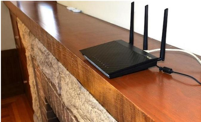
Radio waves travel best through open air, so sight lines are a good clue here: if you can see the router from far away, and from many different angles, you're using it efficiently.
