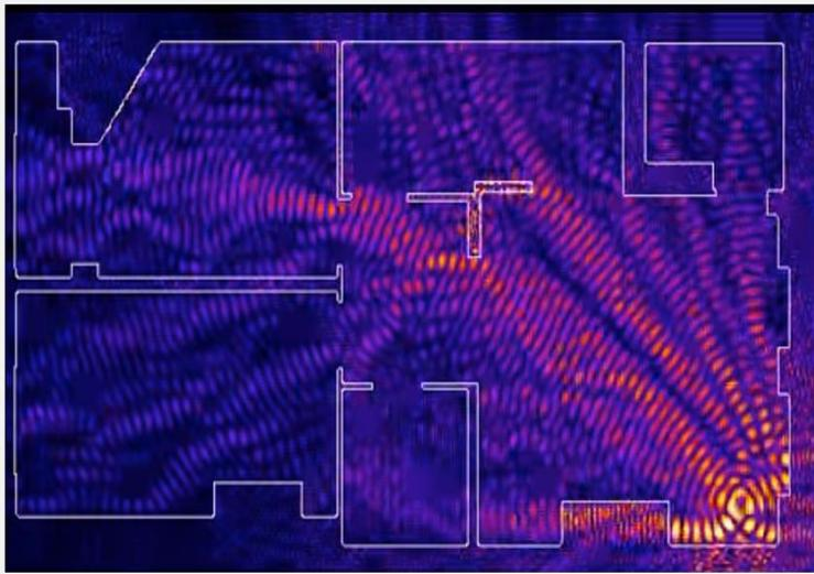
A router sends out signals in all directions, so putting it in a corner of your home (as shown in the diagram) means that much of its signal is wasted.
