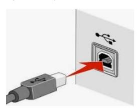
of us know how to connect the standard USB male connector to our computer, but there is more confusion with the other end of that USB cable that attaches into (usually) the back of the printer (see the picture to the left).
