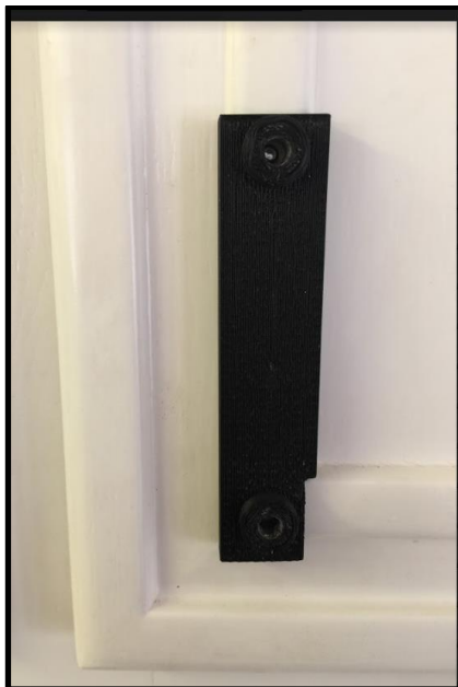
Jig on cabinet door
