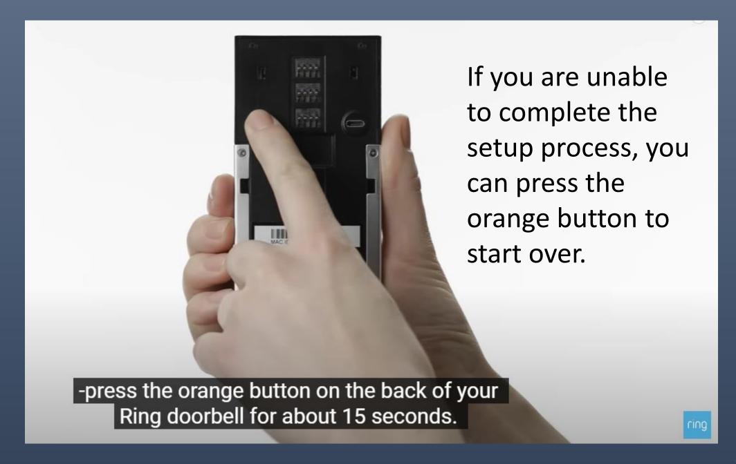
Decide on a location for the Ring Doorbell. If you have an existing doorbell button you can attach those wires to the Ring Doorbell Be aware of the field of vision. The Ring 4 comes with a mounting wedge to angle view
